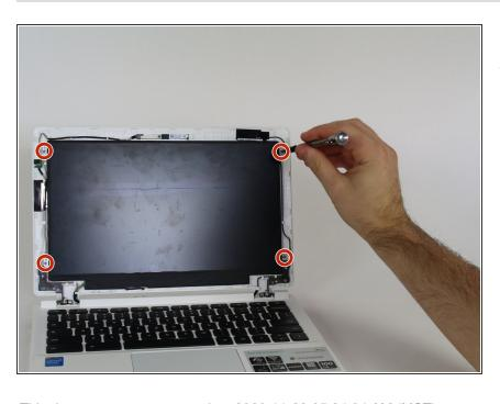
Locate and remove the four 4.2mm screws holding the screen in place by using a Phillips #1 screwdriver.
