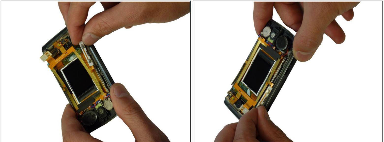
**⚠ Caution:** The side buttons are attached to the ribbon around the display screen. Do not separate the side buttons from the ribbon when removing.
