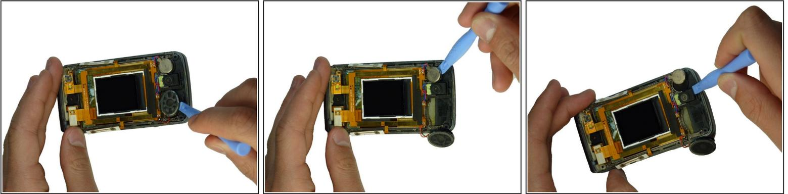
**⚠ Caution:** The wiring on the ribbon connector is delicate. Do not excessively pull on the wires.
