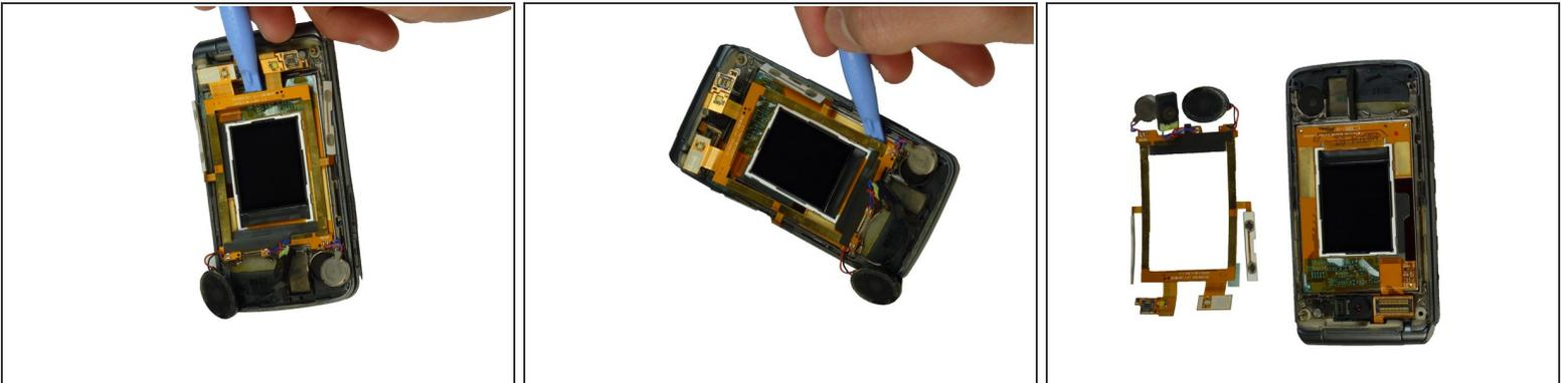
**⚠ Caution:** The ribbon contains important wiring and is glued to the phone. Be careful when removing the ribbon.
