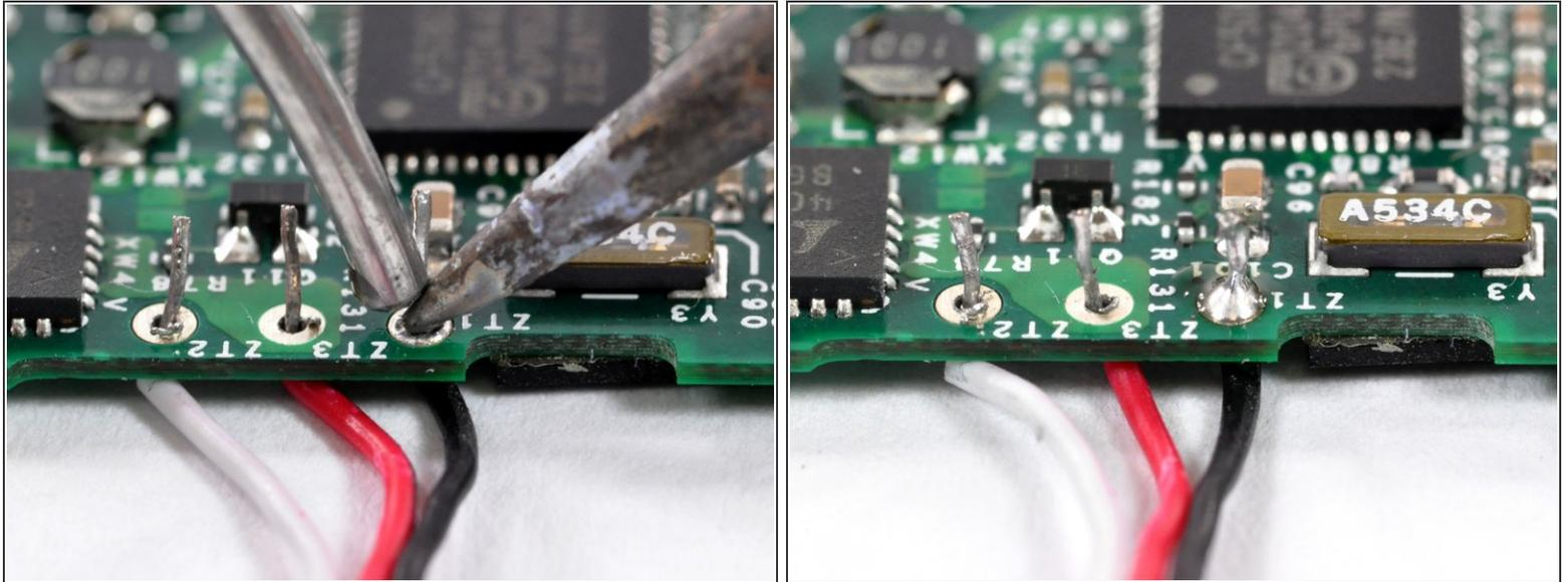
**i** In this step, you will solder the battery leads to the solder pads on the logic board.
