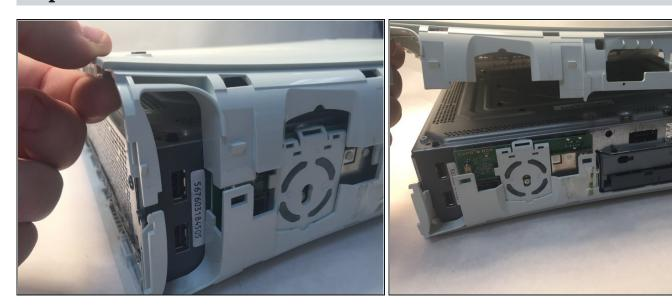
• Unlock clips from the front of the console and take off white hood. Pull hood up to remove it.
