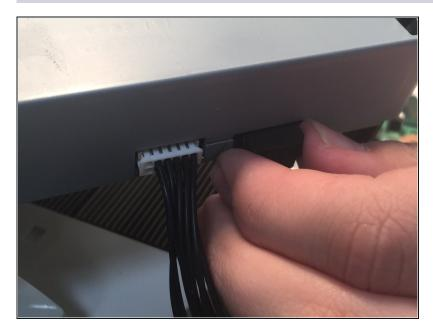
Remove the disc drive removing the output and input plugs.
