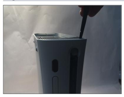
Use a spudger to pry open the top face plate, make sure not to break any of the clips, or the plate itself.
