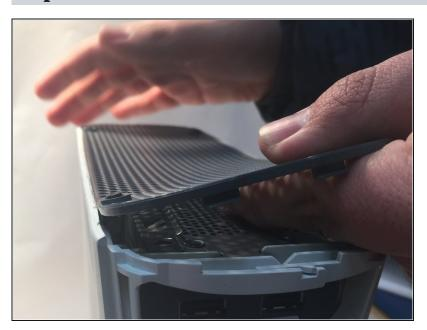
Pry or wiggle off gray end plates from the top and bottom of the console.
