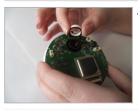
Remove the washers between the lens and motherboard.
