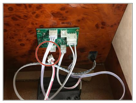
• Unplug motor connection cable from circuit board
