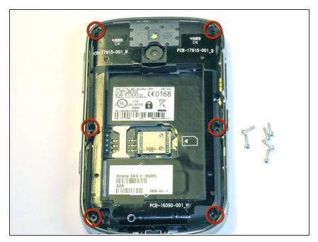
Remove the six 7.0mm Torx screws securing the rear case to the rest of the phone.
