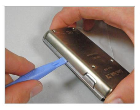
Using a plastic opening tool, lift the metal backing from the front of the device.
