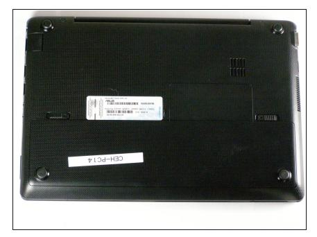
Lay the laptop flat on a hard surface with the bottom facing up and the battery pack on the side closest to you.
