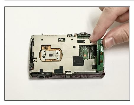
Lift the button circuit board by gently popping it out of its connector.
