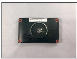
Remove the four screws on the back of the GPS using the T5 Torx screwdriver.
