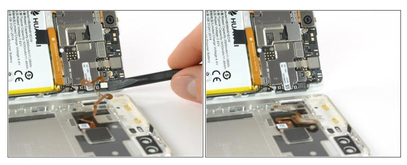
Disconnect the fingerprint sensor using a spudger.
