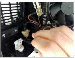
Use a Phillips #0 screwdriver to remove the 1.3mm screw on the black rectangle above the Tip-Over Safety Switch.
