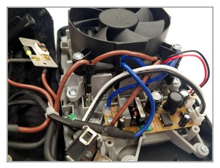
Disconnect all of the blue wires. There should be 3 separate bluewire connections.
