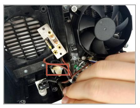
Use a Phillips #2 screwdriver to remove the two 1.7mm screws from the white triangular piece covering the power cord.
