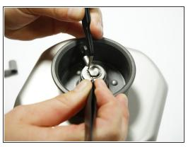
• Flip the bread pan over and locate the "C" shaped clip. Orient the clip so the ends line up with the flat part of the bolt. Using tweezers or "C" clip pliers, pry the clip apart and remove it.
