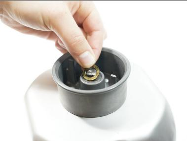
Once the clip is removed, the wing washer and circular washer can be easily removed by hand or tweezer.
