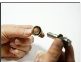
Flip the bread pan over and remove the bolt by hand or plyers if necessary. Remove the seal and replace with a new one. Make sure the seal is oriented the correct direction (refer to the picture)
