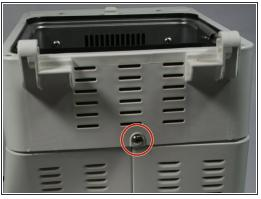
Remove the five 1cm screws that hold the the casing together. There will be two on each side, and one on the back.
