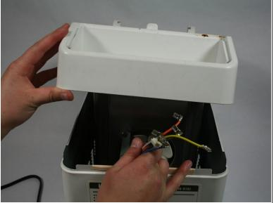
Now you can remove the top part of the assembly off by pulling straight up. Don't forget to gently pull your wires through.
