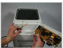
You will then have to disconnect the six wires that connect the motherboard to the device. This can be done by firmly grasping a connector and pulling straight out from the unit. Once all of the wires have been disconnected, set aside the control unit.
