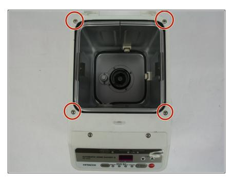
Unscrew the four 1.4 cm screws surrounding the slot for the bread pan.
