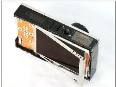
• Pull up the metal frame surrounding the LCD screen starting at the side of the camera.
