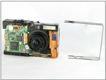
• Slide the metal frame off of the camera on the side that is closest to the flash mechanism.
