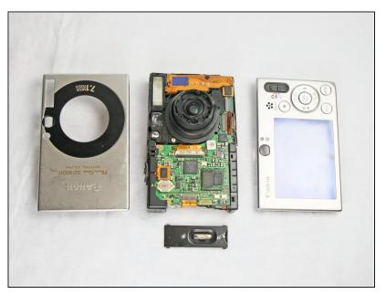
Place the front cover, back cover, and wrist strap mount in a safe place until you are ready for reassembly.
