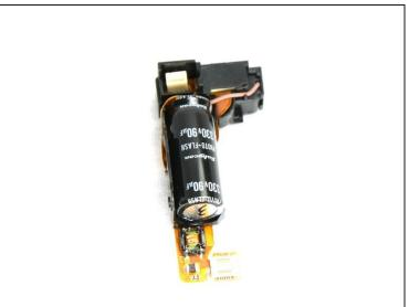
• Pull the flash assembly forward out of the camera to remove it.
