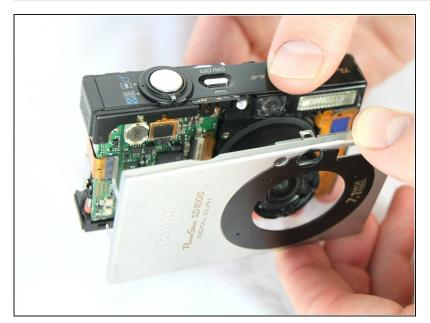
Remove the front cover by gently pulling it away from the camera body.
