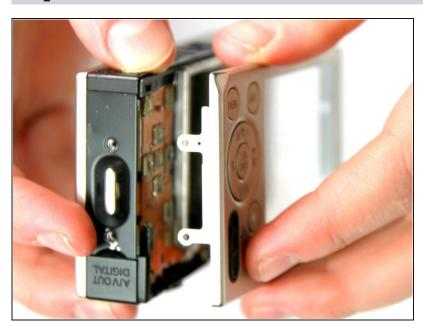
Pull the back panel away from the camera body, starting at the end with the function buttons.
