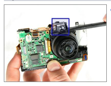
With spudger gently remove the Viewfinder Window that is directly above the lens.
