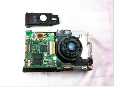
Using the spudger remove the shutter button by prying the small tab on the front side of the camera.
