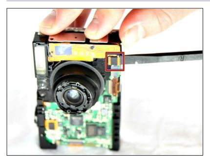
Use the spudger to gently and carefully disconnect the flash assembly ribbon from the black connector lock.
