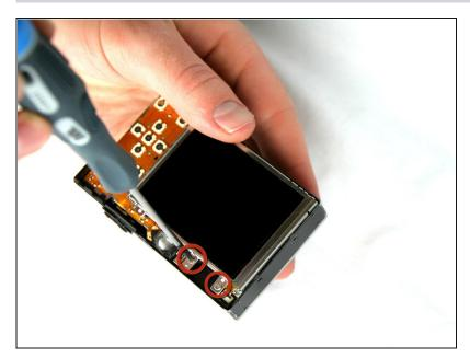
Remove the two 2.4 mm screws located at the top of the LCD panel.
