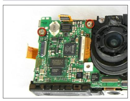
• Remove the two 2.90 mm screws from the motherboard.
