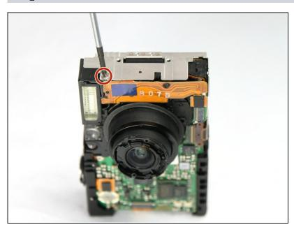
Use a Phillips #00 screwdriver to remove the 2.4 mm screw that secures the flash assembly.
