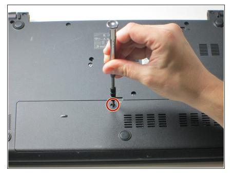
Unscrew the one 2.5 x 8mm Phillips #0 screw from the bottom panel as designated in the image.
