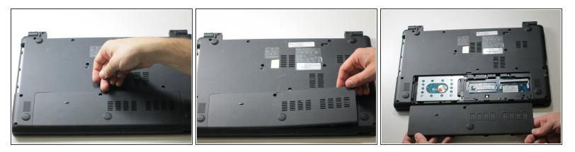
• Remove the back panel by carefully disengaging it around the edges and then pull upwards.
