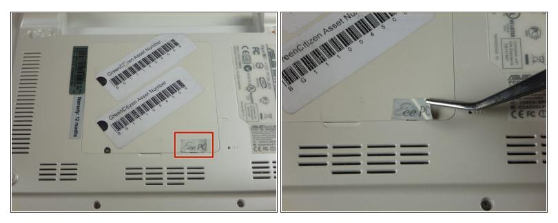
• Remove the sticker from the RAM compartment using a pair of tweezers.
