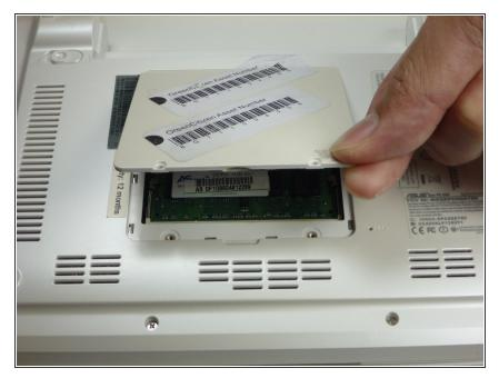
• Remove the back cover by pulling up on the side that had the screws.
