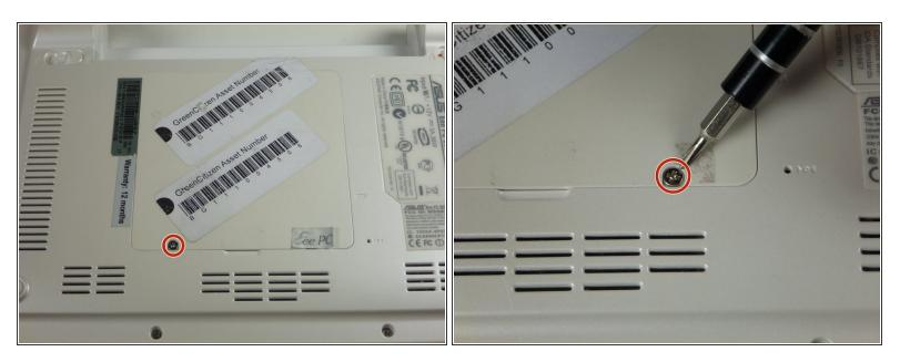
Remove the two 4.8 mm screws using a Phillips #0 screwdriver.
