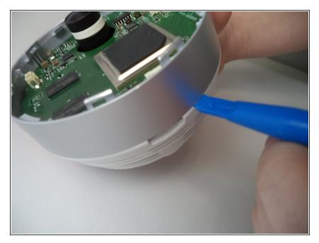
Apply a plastic opening tool to the gray plastic band around the case of the camera. Insert the edge of the spudger between the case of the camera and the gray plastic band.
