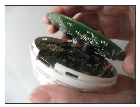
Pull the circular circuit board away from the rest of the device, being careful not to bend any of the pins connecting the two.
