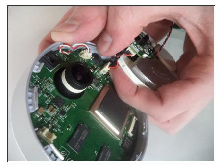
Check to make sure all wires are completely detached from the motherboard.
