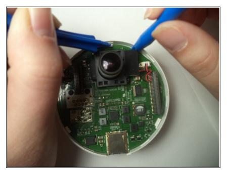
• Press each tab while using a plastic spudger to pry the motherboard up in the location near the tab.
