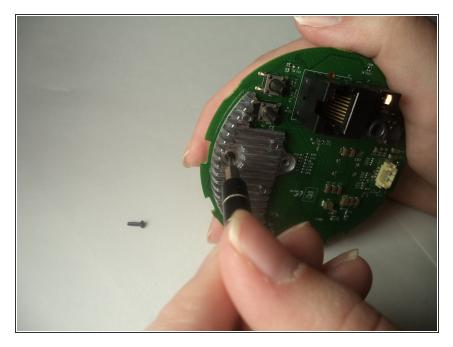
• Using a Phillips #00 screwdriver, remove the screws holding the heatsink to the motherboard.
