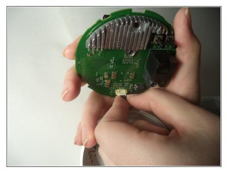
• Unplug the final group of wires from the bottom of the second circuit board and remove the board.
