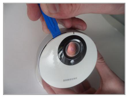
• Locate a small opening around the front panel of the camera.
