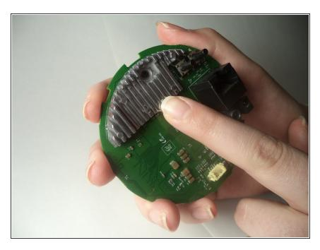
• On reverse side of second circuit board, locate secondary heatsink.
