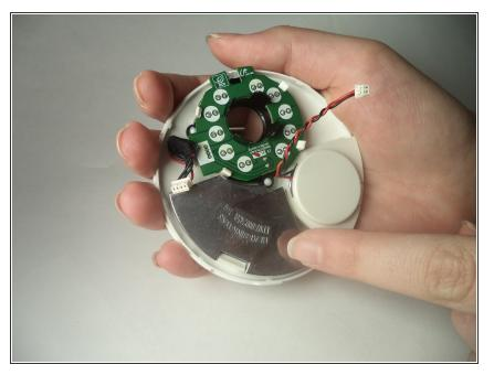
• On inside of front casing, locate heatsink.
