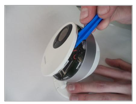
Using a plastic opening tool, apply pressure to various points around the camera to pry open the front panel.
