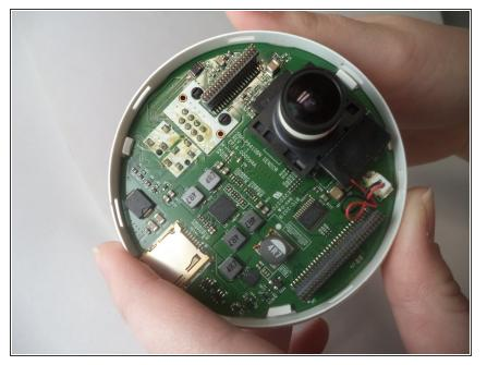
• Locate the three white tabs holding the next circuit board inside the case.
