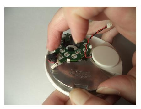
• Using careful force, push in the white tab and pry up heatsink with fingers.
