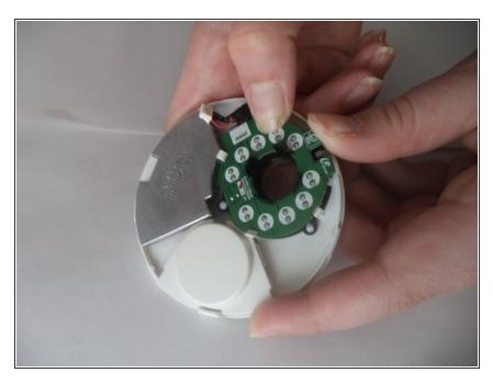
• Push the four white tabs away from the center of the lens housing while pulling the led ring up near each tab.
