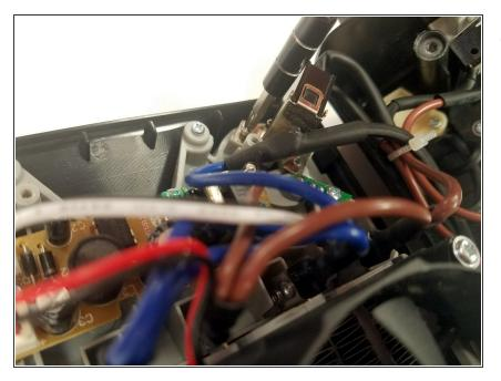
Using a Phillips #1 screwdriver, unscrew the two 7 millimeter screws attaching the power switch to the power button.
