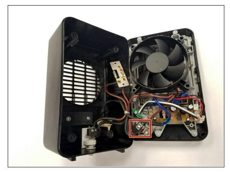
Find the power switch, located inside the heater on the bottom left corner.
