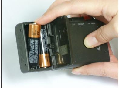
Lift the cover and remove the batteries.
