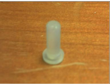
Using a fingernail or other tool, pry out the indicator light (shown on the far left here). You will find that it is actually a small, soft plastic plug
