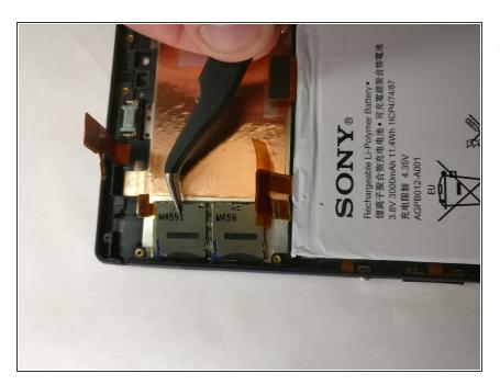
Using the Tweezers, carefully pry the the dual SIM slot off the sticky substance used to hold it down.
