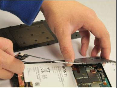
To remove the internal cover, use the plastic spudger tool and pry the cover from the phone as shown in the picture.
