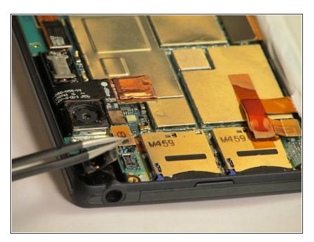
Carefully remove the audio jack by using the tweezers and pull firmly straight out of the motherboard.
