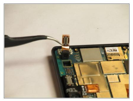
Using the tweezer, carefully pry open the chip for the front facing camera as shown. Then using the tweezer, carefully remove the front facing camera component.
