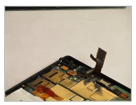
Then using the tweezer, carefully remove the back facing camera component.
