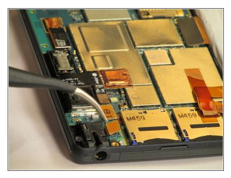
Using tweezer, locate the audio jack as shown and pull out the chip connected to the motherboard.
