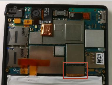
Carefully remove the button circuit connector by using tweezers and gently pulling up.
