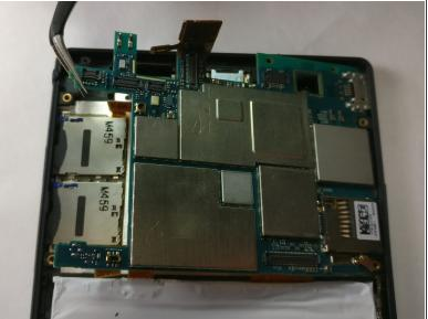
Using tweezers, carefully remove the motherboard by pulling it up and out of the backing.
