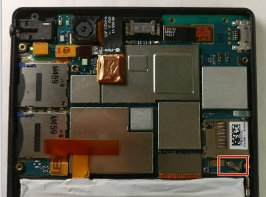
Carefully remove the silver plug by using the tweezers to lift straight up.
