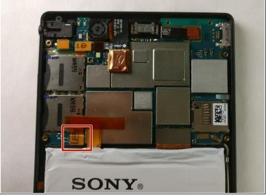
• Using tweezers, locate the battery connector and carefully pull up to disconnect it.
