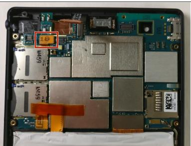
Carefully remove the SIM card connector using tweezers by gently pulling it straight up.
