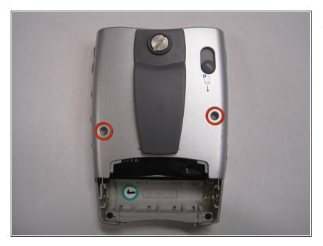
Using a Phillips #00 Screwdriver, remove the two 7.5 mm screws located on the left and right side of the back cover, respectively.
