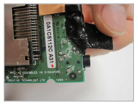
Gently remove the black adhesive tape from the underside of the headphone jack.
