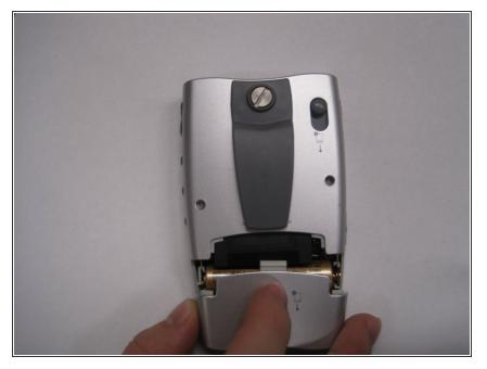
• Using your thumb, slide down and remove the battery cover.
