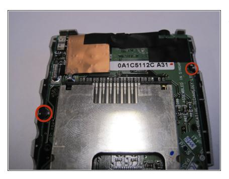
Using a Phillips #00 Screwdriver, remove the two 5.5 mm screws located on the left and right edges of the circuit board.
