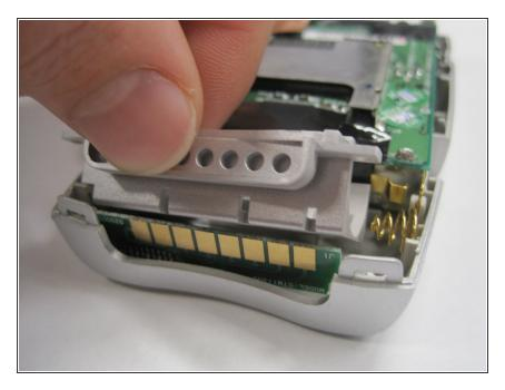
• Using your fingers, carefully remove the battery compartment.
