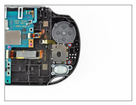
Using a Phillips #00 screwdriver, remove the two blue, 5.0mm screws attaching the left joystick to the back case.
