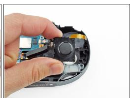
Using a spudger, pry up and remove the left joystick.
