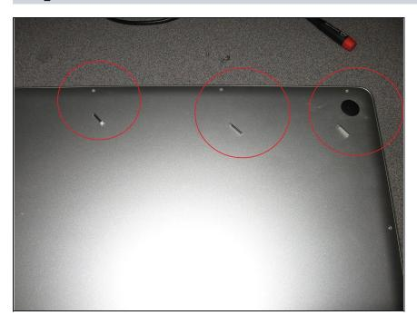
Here are the three larger screws. The smaller ones fit the remaining holes
