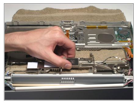
• Grasp the metal heat exchanger and pull up and away from you. You may need to move the inverter cable on the right side of the computer in order to rotate the heat exchanger.
