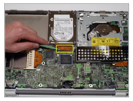
Disconnect the hard drive ribbon from the logic board using a spudger or the tip of your finger, removing tape as necessary.
