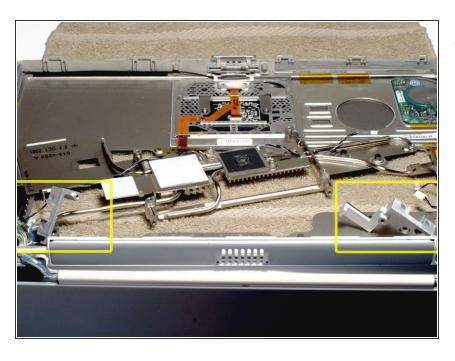
Lift up the metal brackets on either side of the upper case.
