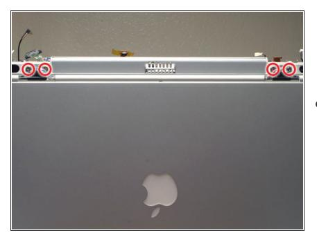
Open the display to a 90 degree angle. Rest the trackpad face down on the work surface and allow the display to hang over the edge. If possible, adjust your chair or work surface height so the display will rest on your legs and the trackpad will lie flat on the work surface.
