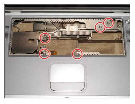
Remove the five silver T8 Torx screws from the metal framework.
