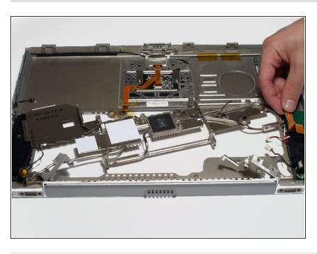
Lift the inverter board out of the computer.
