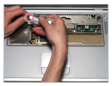
Disconnect the connector cable from the modem.
