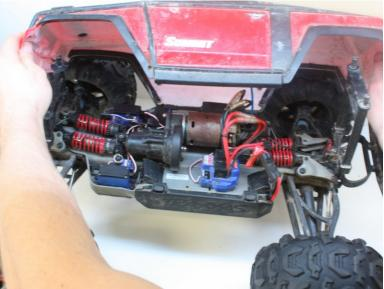
Remove the shell by grabbing it with both hands and lifting upwards.
