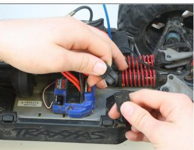
Disconnect the battery from the device by pulling the black plastic connector apart.
