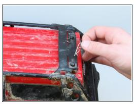
Remove each of the four pins that hold the shell by pulling them from the posts.
