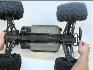
Flip the car on its back to provide access to the steering assembly.
