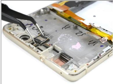
Remove the rubber microphone cover and the earpiece speaker.
