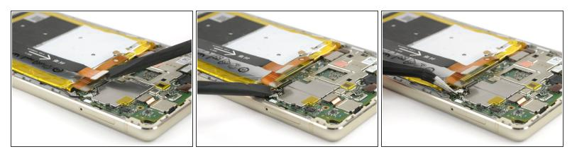
Disconnect the motherboard flex, the battery flex and the antenna cable.
