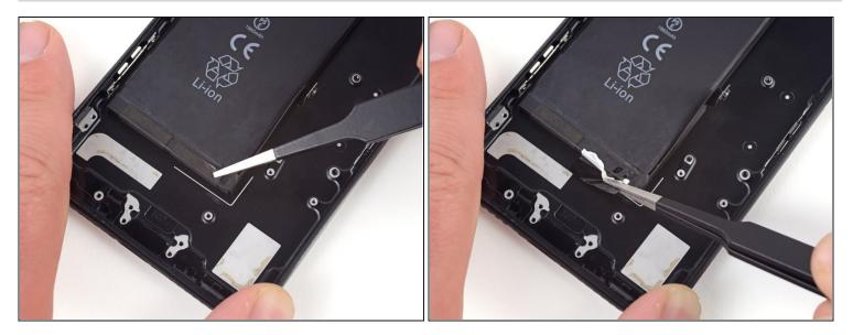
• Use a pair of tweezers with blunt tips to peel back one of the adhesive strips on the lower edge of the battery.
