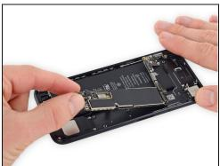
• Lift the battery connector end of the logic board and pull it up and out of the rear case.
