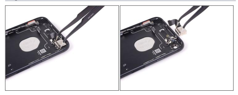
• Use a pair of tweezers to remove the rear-facing camera.
