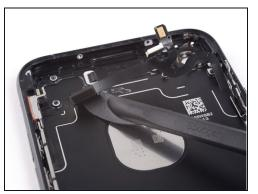
Continue to move the blade of the halberd spudger underneath the power and volume control cable.
