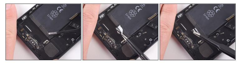
• Use a pair of tweezers with blunt tips to peel back one of the adhesive strips on the lower edge of the battery.
