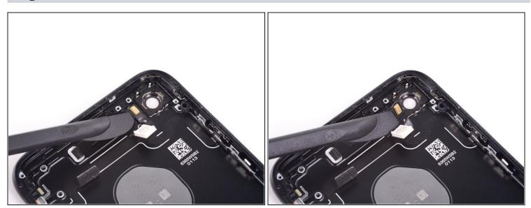
• Use the blade of a Halberd spudger to separate the adhesive holding the microphone to the rear case.
