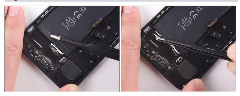
• Use a pair of tweezers with blunt tips to peel back the other adhesive strip on the lower edge of the battery.
