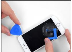
• Re-insert your tool at the lower right corner of the iPhone, and slide it around the corner and up the right side of the phone to separate the adhesive.
