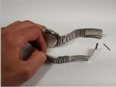
Separate the clasp by pushing in the spring pin.
