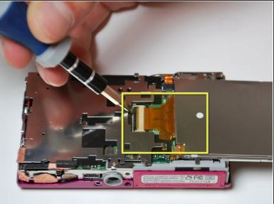
Pull the LCD screen to the left slightly, then lift and flip it open to the right.
