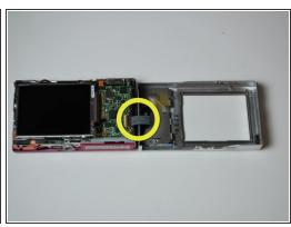
Remove the back by carefully flipping it open to the right side.
