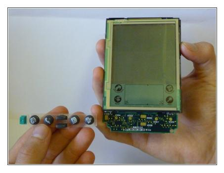
• The keypad is now free to be removed from the rest of the device.
