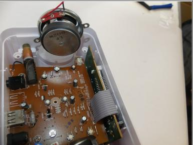
After the speaker cord is removed, pull the speaker straight up and out of the radio.
