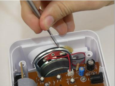
Using a <u>black nylon spudger</u> to carefully break the glue around the outside of the speaker so it can be dislodged.
