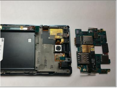
Using a spudger or small prying tool, lift up the motherboard from the chassis of the device.
