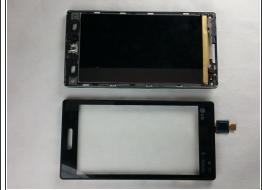
Slide off the connector through the hole of the chassis slowly to avoid damaging it.
