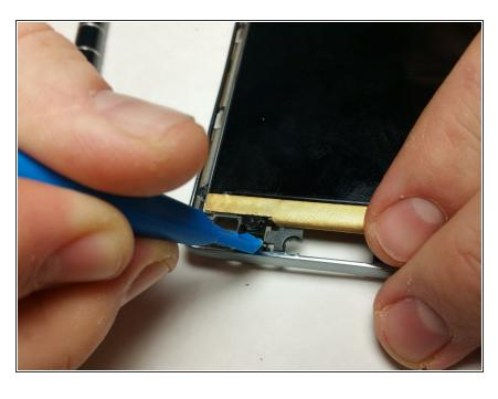
Once the screen has been removed, use a prying tool to lift off the front facing camera. To reassemble your device, follow these instructions in reverse order.
