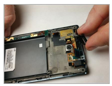
Once the digitizer has been removed, turn the phone face down and remove the plastic housing for the front speaker. It should come off easily.
