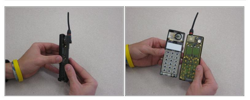
Grab opposite panels of the phone casing and carefully open and pull apart the phone, as shown in the image.
