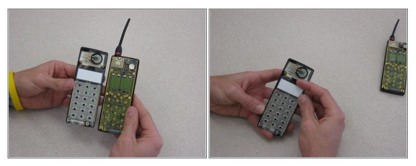
• After removing the battery casing and taking apart the phone casing, the keypad is held in with a plastic skeleton structure as shown.
