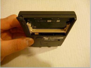
The card fits into the card slot located behind the cover. To remove the card just pull it out of the slot. To reassemble your device, follow these instructions in reverse order.
