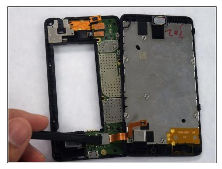
Using the <u>spudger</u> tool, release the top flex ribbon from the light swap package.
