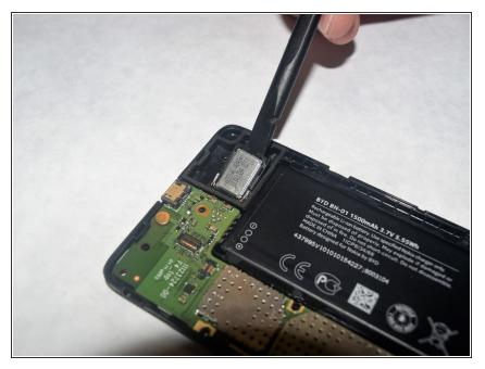
• Use a nylon spudger to pry off the speaker and speaker gasket.
