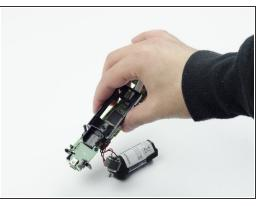
Carefully pinch the plastic sides of the battery slot and lift it (along with the circuit board) from the plastic shell of the move controller.
