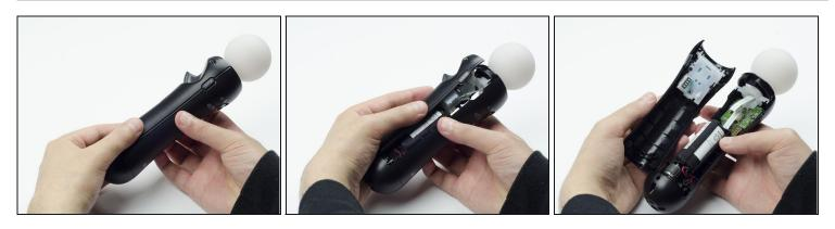
• Pinch the sides of the back panel to remove it and set it aside.
