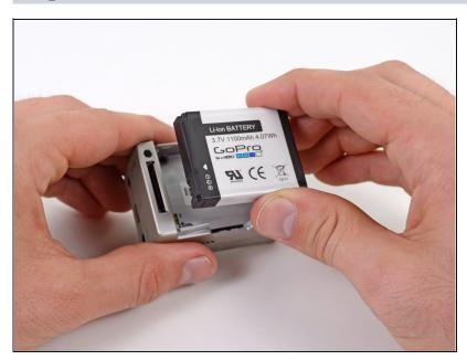
• Remove the battery from the case.
