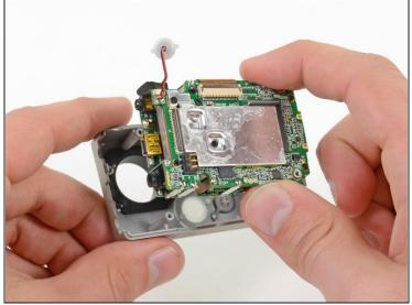
• Gently grab the edges of the motherboard assembly and lift it out of the front case.
