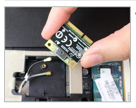
Lift the Wi-Fi card to remove it from the slot.
