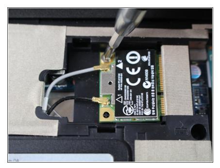
Use the same screwdriver to remove the two 3 mm screws holding the card in place.
