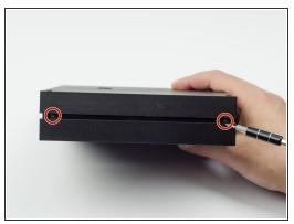
On one side of the console (the side adjacent to the fan vent), there will be two 6 mm screws.
