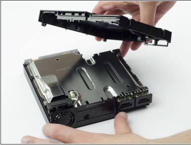
With the plastic opening tool, carefully pry the console shell panel free and lift it away.
