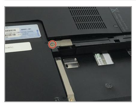
Use a Phillips screwdriver with a PH0 head type to unscrew the indicated 5.5mm screw.
