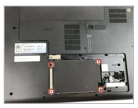
Use the screwdriver to unscrew the four 5mm screws holding down the hard drive.
