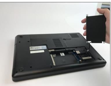
Use plastic opening tools to lift up the hard drive. Set aside the hard drive without disconnecting the wire.
