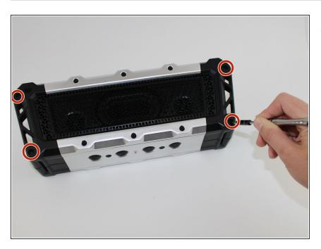
Remove four 3 mm screws using a 3 mm Hex screwdriver.
