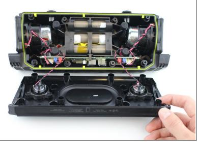
Carefully untangle the wires that connect the speaker to the motherboard.
